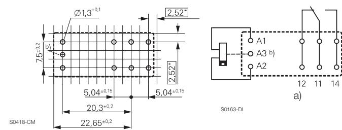
\*) With the recommended PCB hole sizes a grid pattern from 2.5mm to 2.54mm can be used.
